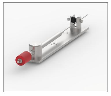
The GEO-DW300 Wire Extensometer is designed to monitor the changes in distance between two anchor points and is complete with vibrating wire displacement transducer. A stainless steel wire connects the transducer to the opposing anchor.
