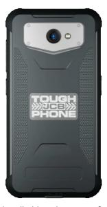
The JCB Toughphone is used as a handheld readout to configure and collect Portable Inclinometer data using the IncloPRO purpose-designed app.
